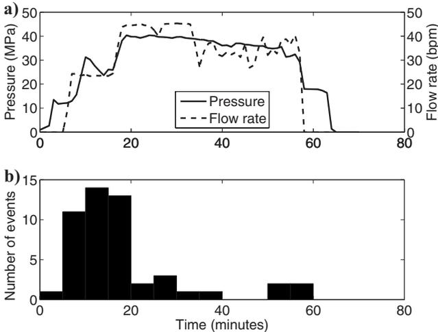
Figure 4. (a) Surface injection pressures and flow rates during CO<sub>2</sub> injection. (b) Rate of microseismicity (bpm = barrels/minute).
