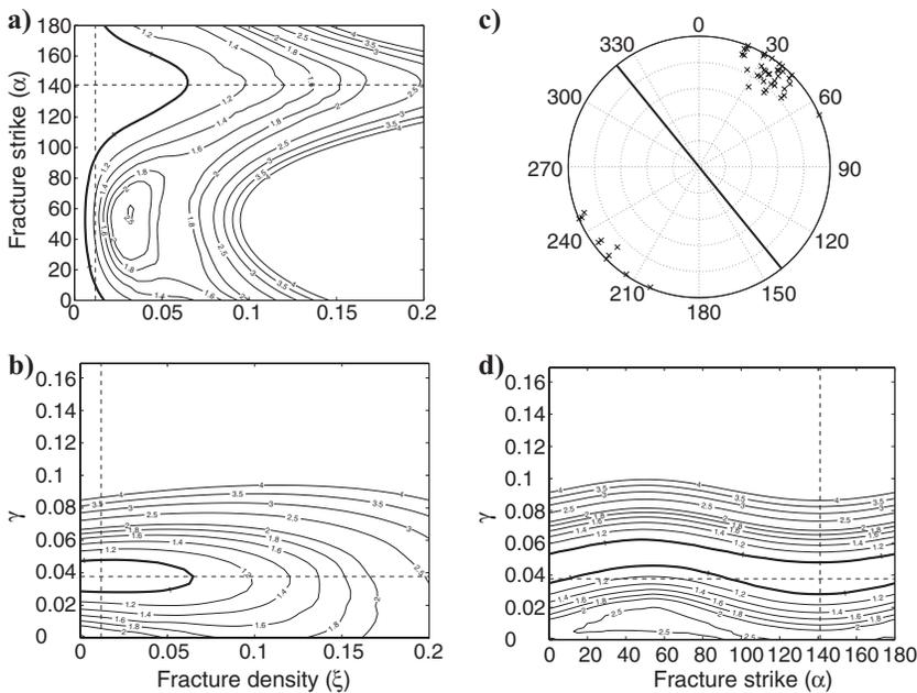
Figure 10. Shear-wave-splitting inversion results for CO<sub>2</sub> injection in the same format as Figure 9. Although the fracture density is less than for water injection (Figure 9), there is overlap between the 90% confidence intervals.
