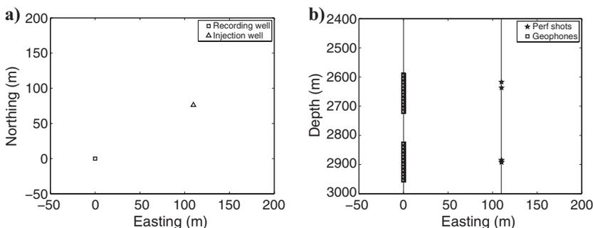
Figure 1. (a) Map view and (b) cross-section plots, showing injection depths and recording geophones for both stages of fracturing. The upper shots and receivers in (b) are for the CO<sub>2</sub> injection stage; the lower shots and receivers are the water stage.
