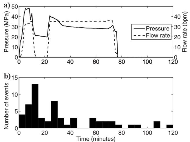
Figure 2. (a) Injection pressures (at surface) and flow rates during water injection. (b) Rate of microseismicity (bpm = barrels/minute).
