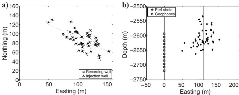
Figure 5. (a) Map and (b) cross-section views of event locations recorded during CO<sub>2</sub> injection. The recording well is at (0,0) and the injection well is marked. The error bars indicate the one-standard-deviation confidence interval. The events are located to the northwest and southeast of the injection point and in cross section extend well above the injection point.
