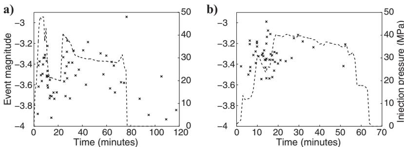
Figure 6. Surface injection pressures (dotted line) and event magnitudes (crosses) through time for (a) water and (b) CO<sub>2</sub> injection. There appears to be correlation between event magnitudes and injection pressures during both stages. Injection pressures and event magnitudes are similar for both stages.
