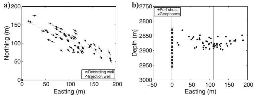
Figure 3. (a) Map and (b) cross-section views of event locations recorded during water injection. The location of the recording well is at (0,0), and the injection well is marked. Error bars represent the one-standard-deviation confidence interval (in some cases, these are smaller than the dots plotting the locations). The events are located northwest and southeast of the injection well, along a strike of  $\sim 120^\circ$ , and in cross section are close to the injection depth.
