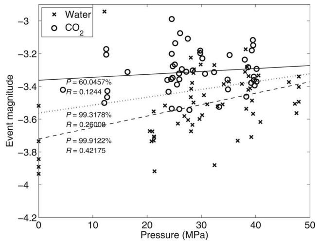
Figure 7. Event magnitudes as a function of the pressure when the event occurs. The events during water injection are marked by crosses; those during CO<sub>2</sub> are marked by open circles. The best-fit lines (dashed = water, solid = CO<sub>2</sub>, dotted = combined), correlation coefficients, and statistical significances are marked.
