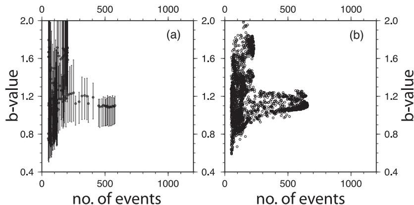
**Figure 6.** Relation of  $b$ -values to the number of events for SRC2008 using the KS-test with a maximum-likelihood method (see supplementary figures for other calculation approaches and catalogues). (a) Along-arc  $b$ -value versus number of events. (b) Grid-search  $b$ -value versus number of events. The uncertainties in  $b$ -values have been omitted for clarity.
