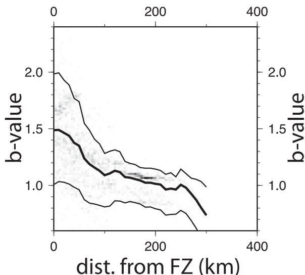
**Figure 10.** Relationship of  $b$ -values to the distance from the nearest fracture zone for SRC2008 using the KS-test with a maximum-likelihood method (see Figs S13 and S14 for other calculation approaches and catalogues). The density of the results is shown with grey shading, the average  $b$ -values (bold line) and their uncertainties (fine lines) were calculated in 10 km steps. The smaller the distance from a fracture zone the greater the  $b$ -value.
