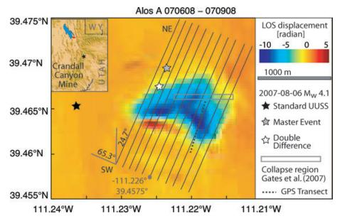
Figure 1. ALOS Interferogram showing LOS displacement in radians (1 radian = 11.8 cm). 11 profiles (black lines) spanning the deformation region capture the gradient of deformation from southwest to northeast ( $24.7^{\circ}$  cw from north) and are used to calculate the mean 2-D deformation (Fig. 2). The plot also shows the three different epicentre locations for the 2007 August 6 seismic event and the estimated collapse region (rectangle) from Pechmann *et al.* (2008).
