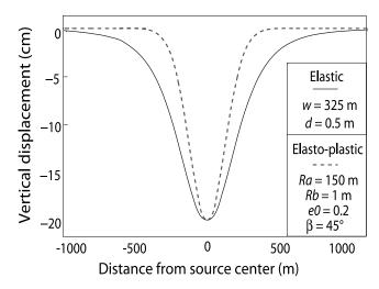
**Figure 7.** Comparison of width of subsidence trough from elastic collapse model and elasto-plastic collapse model. The source depth (600 m) and horizontal extent of the source are the same in both models. The remaining model parameters are chosen with similar values to cause the same subsidence amplitude. It can be seen that the wedge boundaries in the elasto-plastic model limit the lateral extend of the subsidence trough, causing higher deformation gradients.
