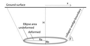
**Figure 6.** Schematic illustration of the elasto-plastic collapse model, modified from Loganathan & Poulos (1998). The elliptical source geometry is defined by its major axis Ra in x-direction and minor axis Rb in z-direction. The lateral extent of the subsidence trough is controlled by angle of the wedge boundaries from horizontal  $(\beta)$ . The area loss of the cavity cross-section is defined by strain  $\varepsilon$  (see eq. 6).
