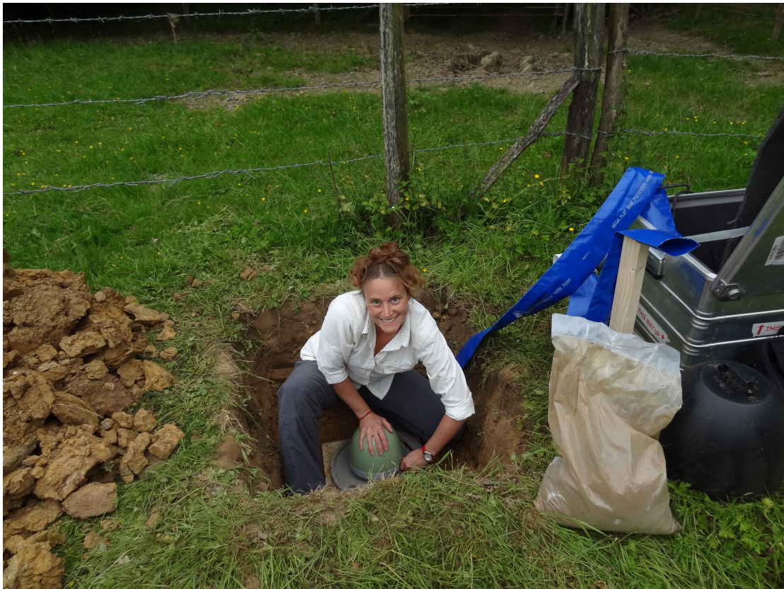
Figure 2: Seismometer deployment at BA03. The green dome-shaped object is the sensor resting on an insulating base laid on the levelled paving slab at the bottom of the hole. The blue tubing is the firehose through which all cables are threaded to protect them from rodents. The grey box is the Zarges case containing the batteries and the data logger.
