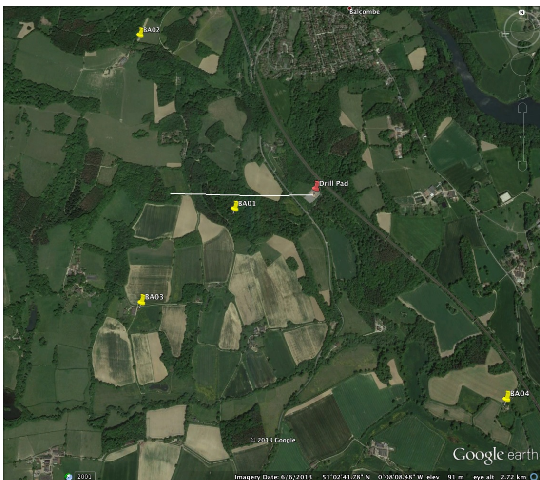
Figure 1: Area map of Balcombe, the seismic array (yellow pins labelled BA01 – BA04), the drill pad (red pin) and the proposed drill line (white line). Of specific interest is the railway line that snakes from the centre top of the map, to the West of Balcombe village and to the East of the drill pad, exiting the map to the East of BA04. BA04 was located close to the line to monitor train noise.
