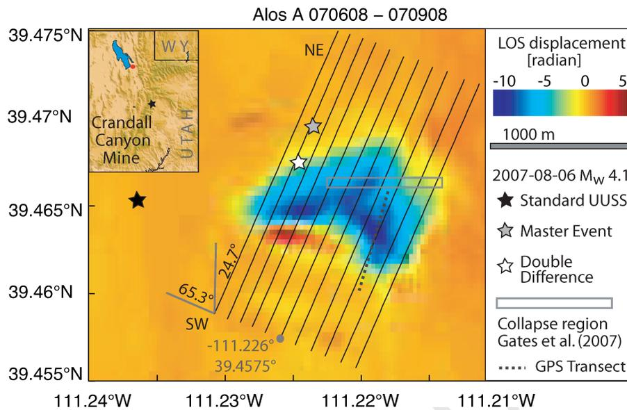
**Figure 1.** ALOS Interferogram showing LOS displacement in radians (1 radian = 11.8 cm). 11 profiles (black lines) spanning the deformation region capture the gradient of deformation from southwest to northeast ( $24.7^\circ$  cw from north) and are used to calculate the mean 2-D deformation (Fig. 2). The plot also shows the three different epicentre locations for the 2007 August 6 seismic event and the estimated collapse region (rectangle) from Pechmann *et al.* (2008).
