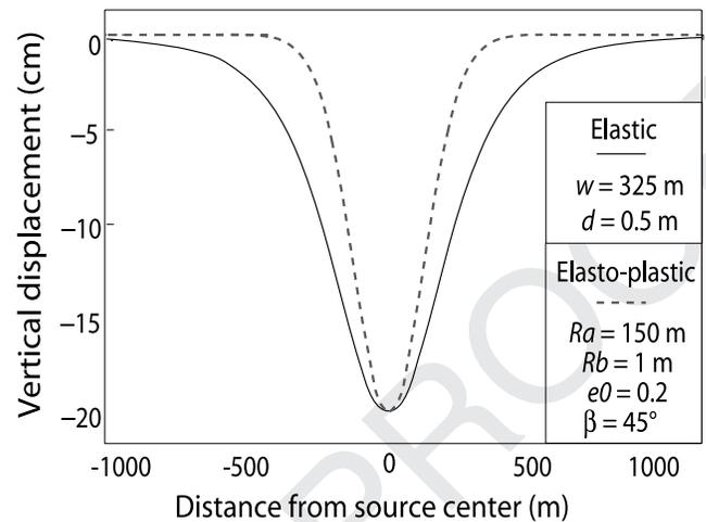
**Figure 7.** Comparison of width of subsidence trough from elastic collapse model and elasto-plastic collapse model. The source depth (600 m) and horizontal extent of the source are the same in both models. The remaining model parameters are chosen with similar values to cause the same subsidence amplitude. It can be seen that the wedge boundaries in the elasto-plastic model limit the lateral extent of the subsidence trough, causing higher deformation gradients.
