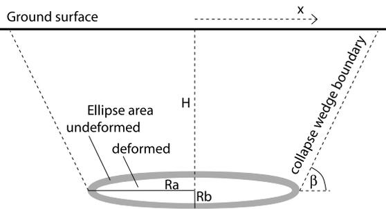
**Figure 6.** Schematic illustration of the elasto-plastic collapse model, modified from Loganathan & Poulos (1998). The elliptical source geometry is defined by its major axis  $Ra$  in  $x$ -direction and minor axis  $Rb$  in  $z$ -direction. The lateral extent of the subsidence trough is controlled by angle of the wedge boundaries from horizontal ( $\beta$ ). The area loss of the cavity cross-section is defined by strain  $\varepsilon$  (see eq. 6).
