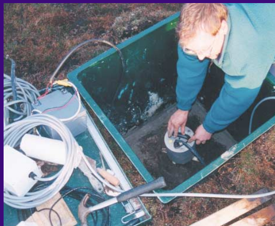
4: Station pit design. Instruments are housed in a fibreglass box mounted on a poured cement pad. The seismometer sits on the concrete. The data logger, battery and GPS antenna are housed on a shelf above the seismometer. Dave Francis is shown installing the station at Arisaig, Scotland.
